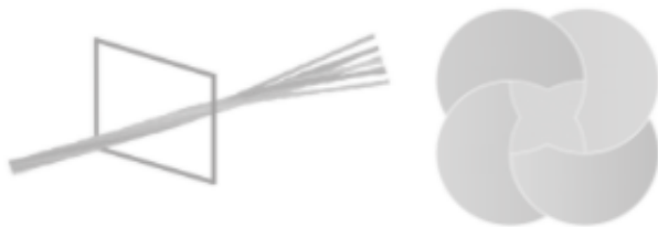
Figure 4. A transversal cut of a 5-thread rope.
